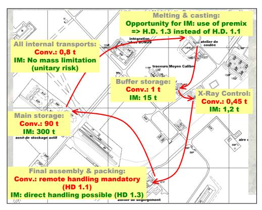
FIGURE 3: Example of industrial fluxes in Nexter's plant, the maximum acceptable weight of explosive is indicated for each workshop with comparison between conventional and IM shells.
