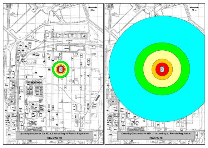
FIGURE 2: Example Regulatory Constraints Reductions for EURENCO's Sorgues Plant "For 10 times less of Net Quantity Explosives, Quantity-Distances are 6 times larger for detonation risk"
